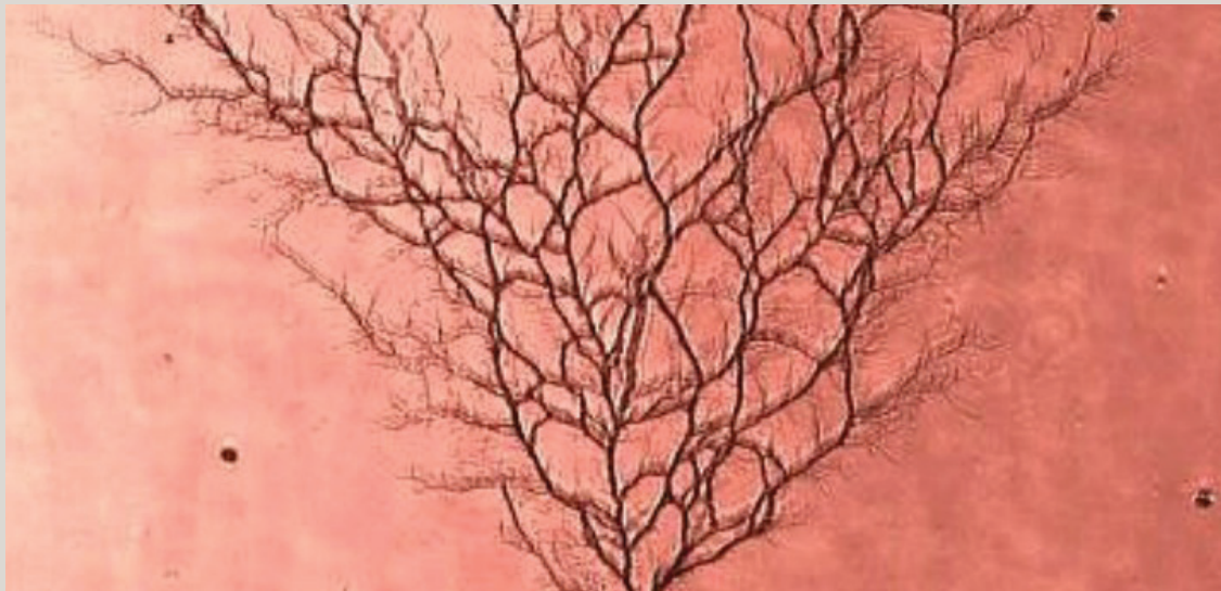
Micro- and nano-fluidic channels in polydimethylsiloxane (PDMS) photographed through an epifluorescence microscope. Photo: JNS.org.
